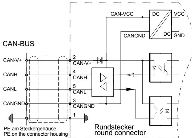
The BUS interface is galvanically isolated from the internal device voltage.
