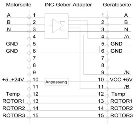
The device input for the incremental counter signals requires the push-pull counter pulses for a reliable detection.
