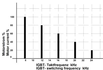
Automatic current reduction depending on the pulse frequency
