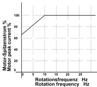
Automatic current reduction depending on the rotation frequency (motor speed)
