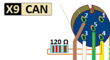
Terminating resistor at both ends of the bus line > 120 Ohm between the CAN-H and CAN-L.
