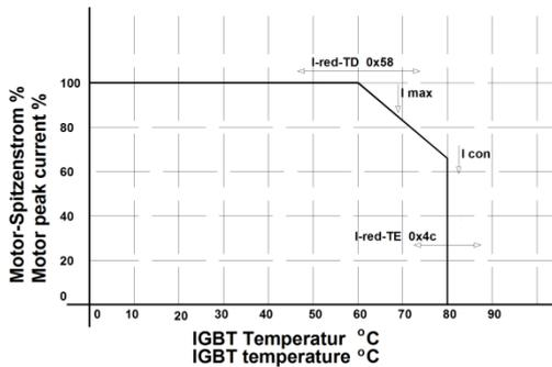
Programmable current reduction depending on the IGBT module temperature. Starting temperature of the reduction I-red-TD 0x58
