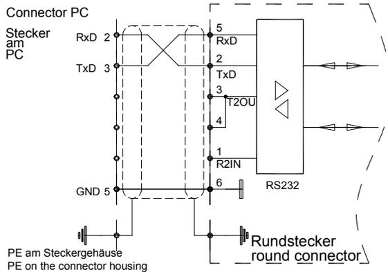
The serial interface is galvanically connected with the device zero (GND/AGND).
