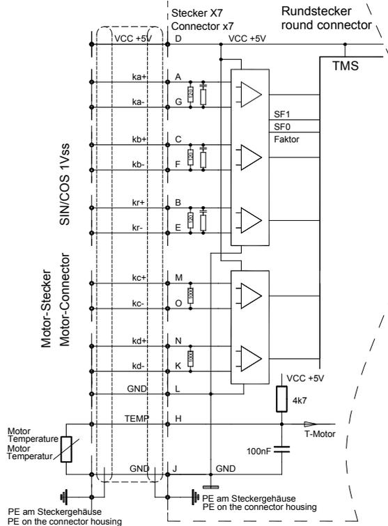
Incremental encoder (encoder) with 2 analog, sinusoidal counter tracks and 1 zero track plus 2 commutating tracks. Differential signals 1 Vss
