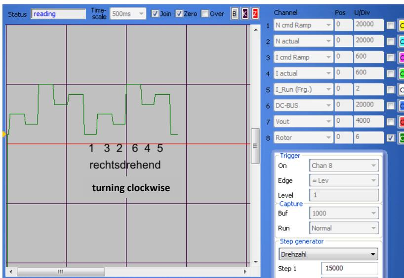
The correct sequence of the rotor signals with a motor turning clockwise is 1, 3, 2, 6, 4, 5.
