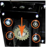
Figure 22: Release toothed belt tension
