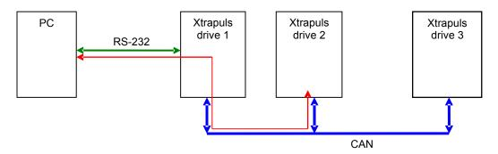
The **Xtrapuls** drive supports Node ID setting by GemDriveStudio software: menu "Tools", sub menu "Node ID setting". Node ID value must be unique for each drive connected on the fieldbus. Node ID range is from 1 to 63.
