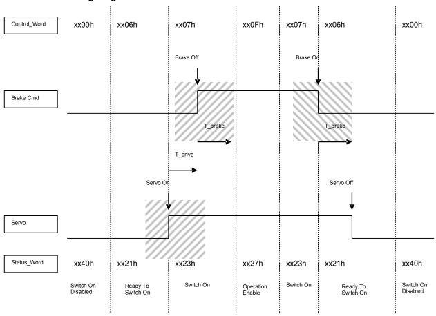
T\_brake: Motor Brake Reaction Time
