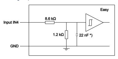
\*) From serial number 11420004, the capacitor value is 10 µF for the IN4 input only, in order to support safety relays with test pulse output (for short-circuit detection).
